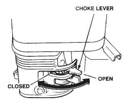
Figure 13. Choke Lever
